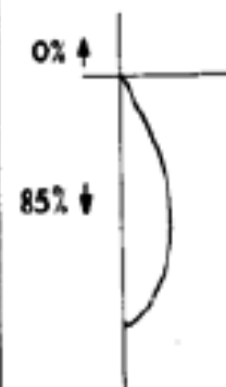
R-40 flood with specular anodized reflector skirt; 45° cutoff
